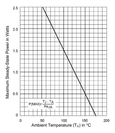
FIGURE 5 Steady-State Derating Curve for Free-Air Mounting ( $R_{\theta JA} = 50$  °C/W)
